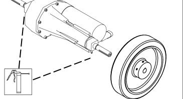
**CAUTION:** Do not use pressure washers to clean sealed gear boxes or bearings. If it becomes necessary to clean under machine with a pressure washer; Ensure all items noted are relubricated
